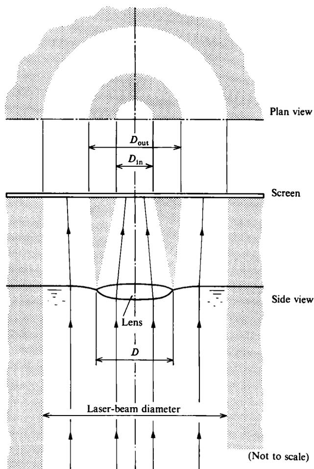
FIGURE 2. Illustrative diagram of geometric relation between a lens on the water surface and its image on the screen.
