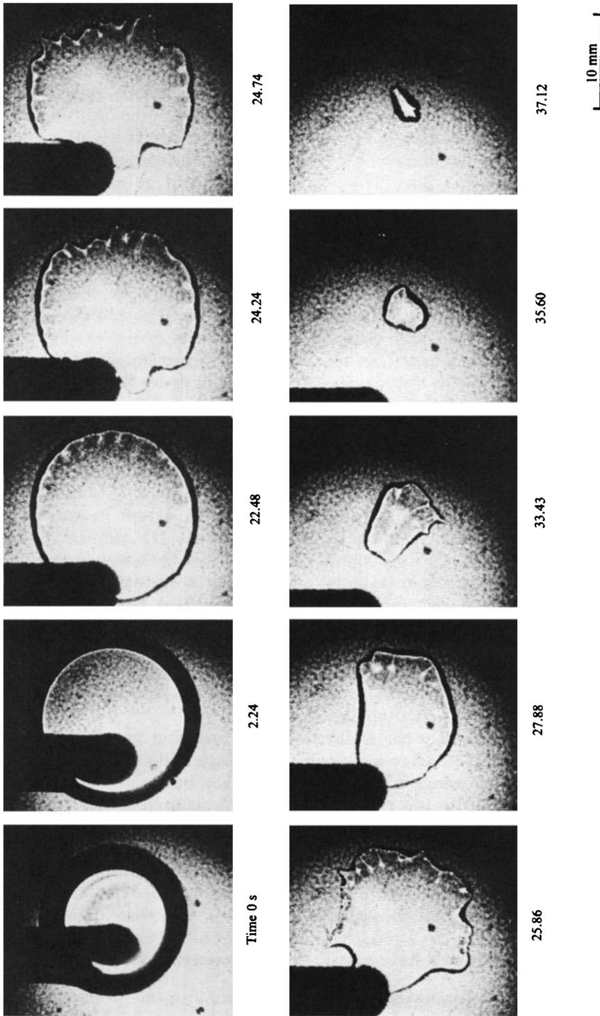
FIGURE 7. Shadowgraphs of an evaporating lens. Run F-16 (see figure 3).
